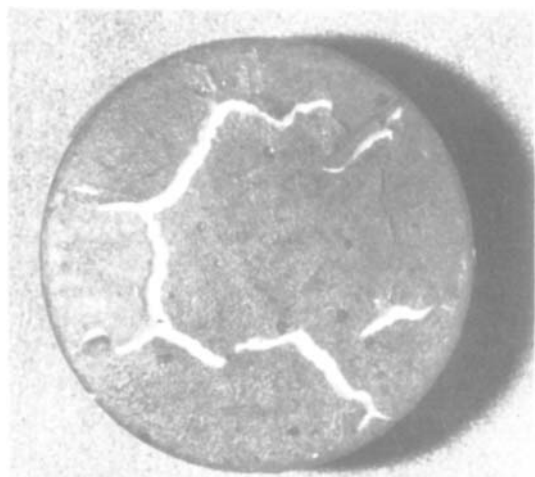
FIG. 1. A cracked film on a film coated tablet.
